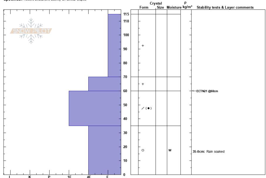
Notes: Pit dug on below treeline wind protected road cut where loose dry avalanche (D1) was intentionally skier triggered from the top. Looking for storm slab. Very quick test pit. Did not use magnification to identify crystal types.
