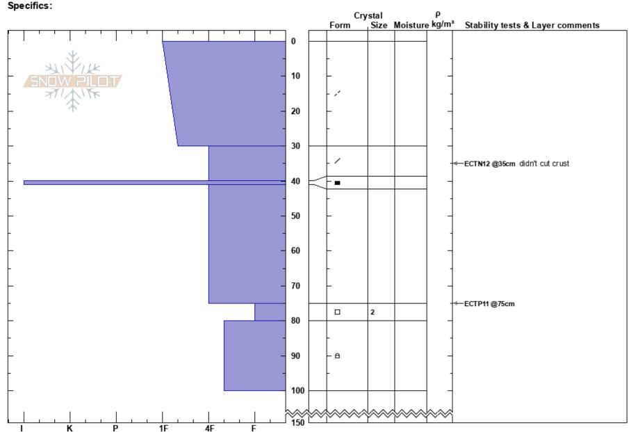
Notes: Cut through the crust (40 cm down) and produced ECPT12 down 75cm. In a separate test, we stopped the cut at the crust and did not get results below the crust. While the crust can support a skiers weight in places, it is not a guarantee and it is safer to assume that an avalanche could be triggered below the crust.
