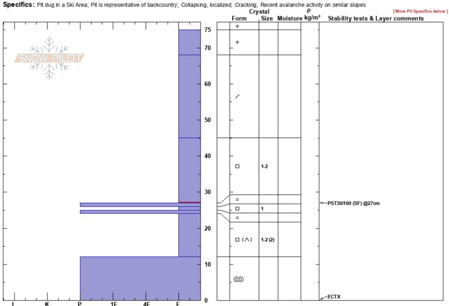
Notes: Lack of slab stiffness so far made stability tests pretty dull. However, in areas with similar structure with more recent wind loading had fairly widespread cracking and collapsing during ski travel. Additional Pit Specifics: Recent avalanche activity on different slopes; Instability rapidly rising
