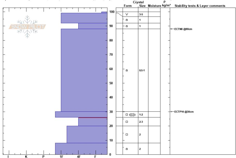
Notes: ECTP14 @30 failed on top of and through decomposing crust (30-26cm). Slab was a drift in the starting zone and very isolated.
