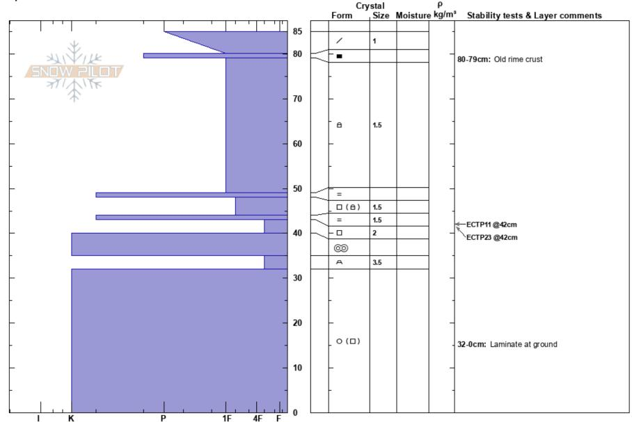
Notes: Variable test results on slopes with same aspect and elevation.
