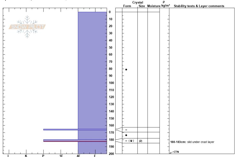
Notes: dug into crown to investigate failed layer, that was the focus ergo not many other data points. Crust layer that it slid on went with the slab. Bed surface is under the crust. HS-AHc-R4-D3-0
