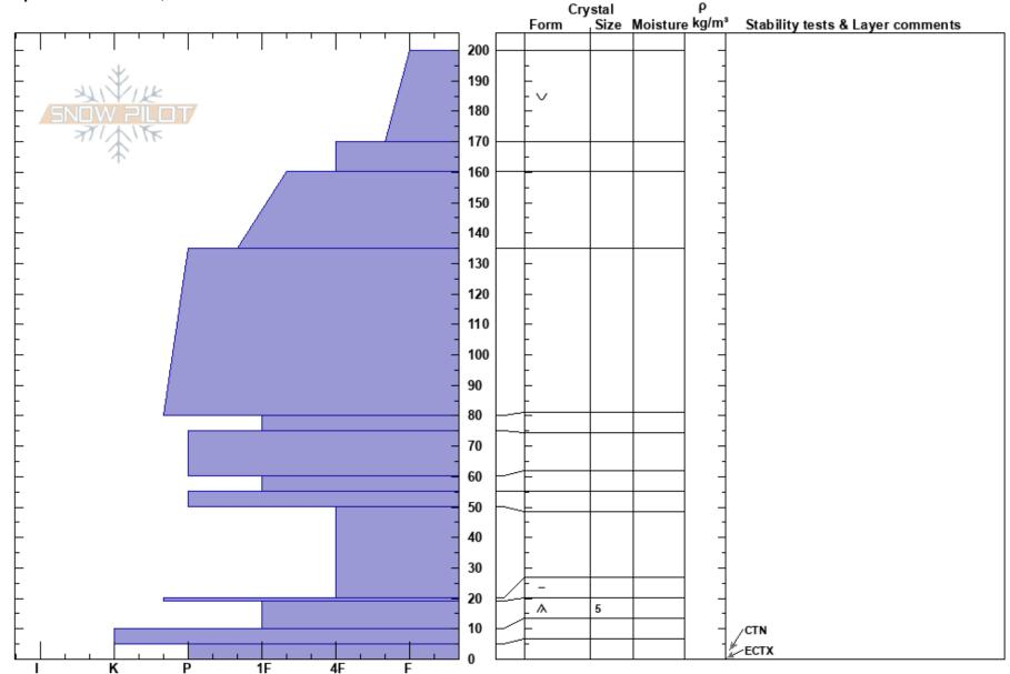
Notes: were able to pull out columns from both tests and they broke at the 1f facets @ 19cm
