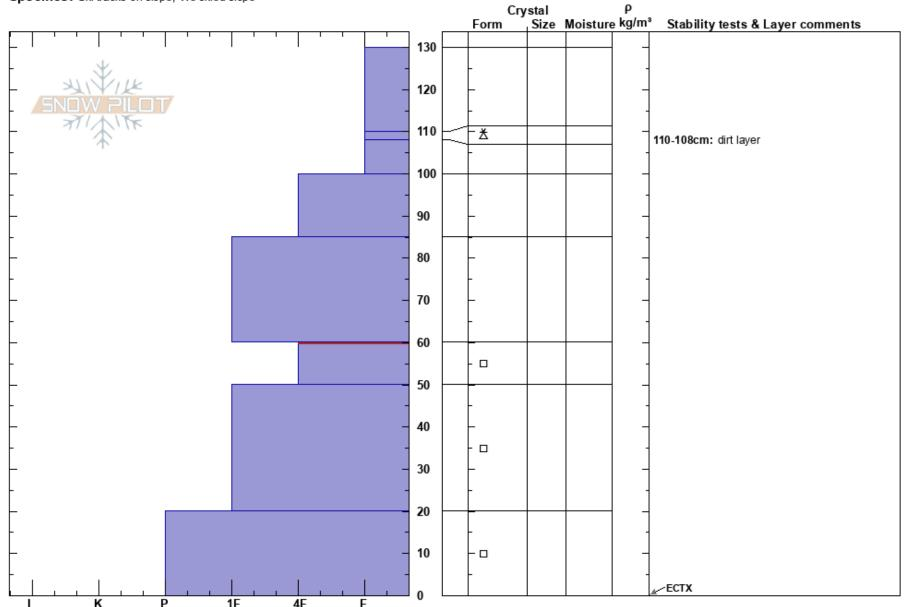
Notes: Winds were SW 16G22 from Reynold's Anemometer. Reynold's north face was scoured in some locations center and loaded in others. High Wind run with max gust of 130mph on Hidden Peak and 61mph at Reynolds. Shovel Tilt test 5 taps PC @108cm (dirt layer)
