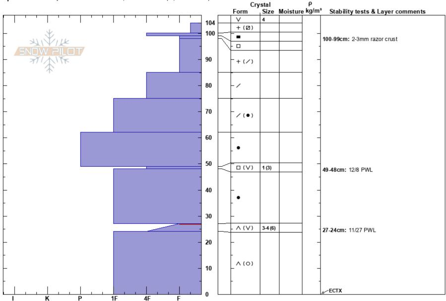
Notes: Crown profile dug 7 days post incident: 100' wide, slope angle 33-37, aspect 270-285. Avalanche failed on both 12/8 (48-49cm) and 11/27 (24-27cm) faceted layers. Stability tests: ECTX x 2, but both tests failed @27cm and propagated with heavy force (kicking shovel). There was very little untracked snow to perform tests, and the column sites were too close to the crown (<1m) to yield valuable results.
