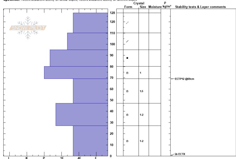
**Notes:** Pit dug on a road across a steep hillside which was drifted over. Slope is flat, but snow surface is 22degrees. Snow depth varied from 120-250cm over about 5m. ECTP12 was in shallower area, and snowpack was much stronger as we dug into the deeper part of the drifted slope (ECTX). Profile was taken in an average depth of where our tests were performed. ECTP12 broke in a layer that was softer and more faceted where it was shallower.
