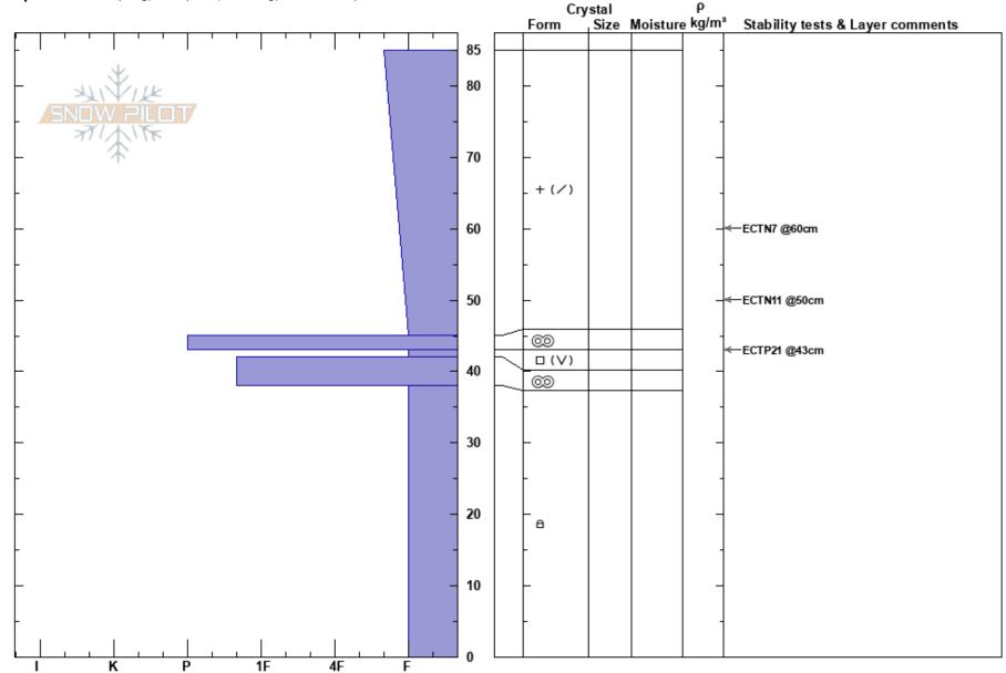
Notes: New snow skied upside down. 48 hr snowfall ~40cm. Propagation in pit below first crust in crust-facet sandwich. Extensive cracking on E-SE-S aspects. Collapsing on all aspects at lower elevations. This storm doubled the snowpack on S aspects.
