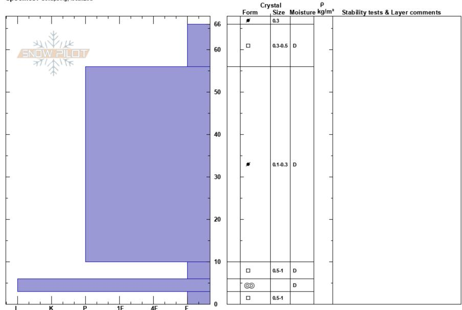
Notes: Attempted 2 ECTs but the mid-pack was too hard for the cord to cut all the way to the bottom. Both tests had the cutting cord get stuck ~10cm from the bottom of the wind-packed mid-layer. Performed tests anyway and both times there was failure on the ground across the block and a fracture in the mid-pack.
