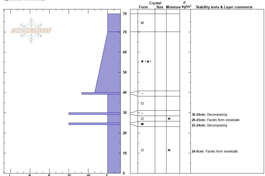
Notes: Widespread surface hoar and near-surface faceting, particularly on north aspects. Much of the top 10-20 cm of the snow is beginning to facet. The crust layers near the base were all decomposing. Basal facets becoming moist -- can form into snowballs.
