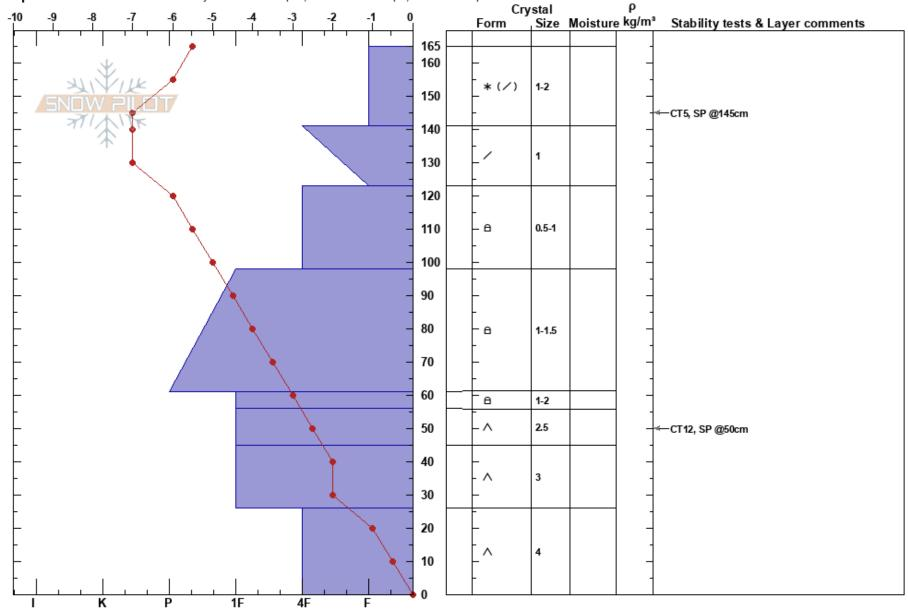
Notes: This was a deep snow pit with the top half displaying many layers of weakness from the CT test, ranging from 25cm down to 150cm. However, the basal layer of the snowpack was hollow facet cups and were supprisingly not reactive with any of the stability tests. We found rounding facet particles mostly in the middle of the snowpack displaying some healing and re-bonding characteristics.
