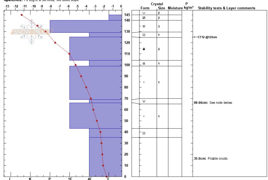
Notes: Layer 7 is made up of an unusual form: 5mm-long needle-like crystals. Possible surface hoar that has been rain affected. This layer is very distinct and very fragile.
