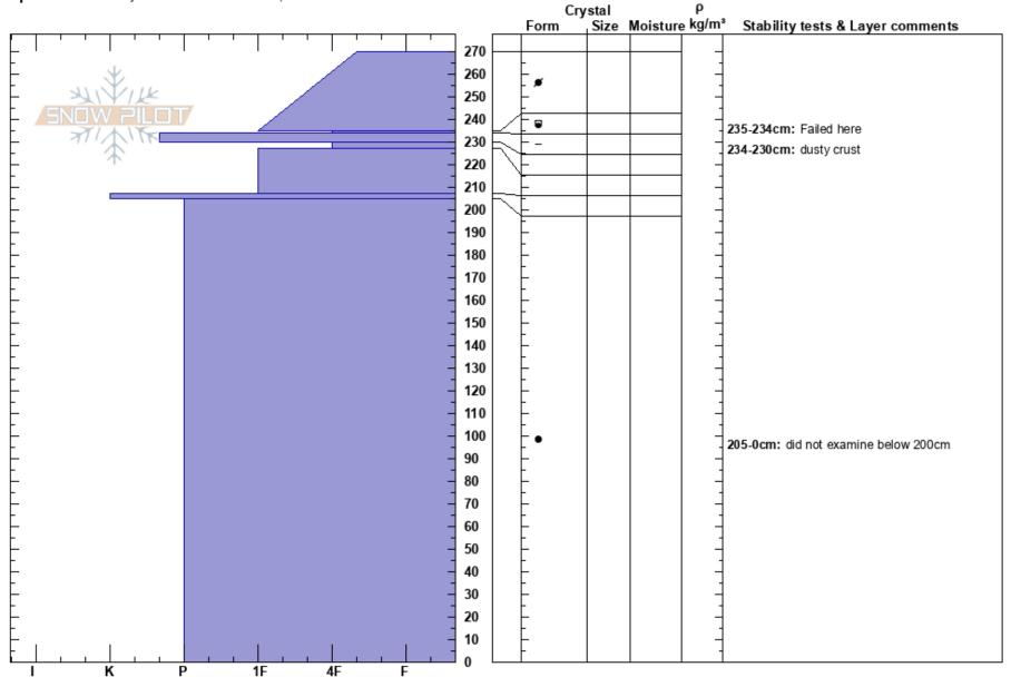
Notes: Quick crown profile. In this area the slab failed on the new/old snow interface. We did not notice the crust sandwich structure that we found near the west flank of the avalanche.
