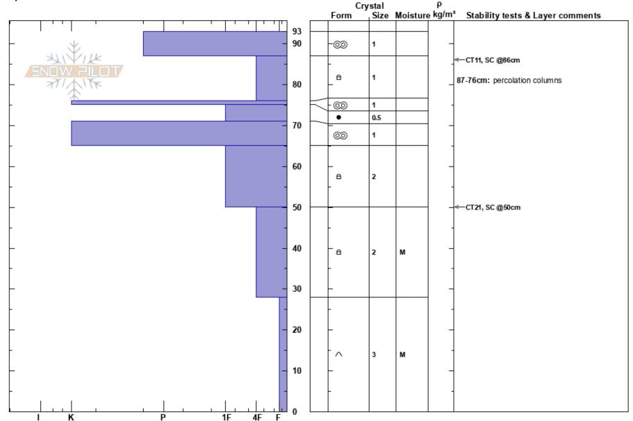
**Notes:** Currently very stable due to multiple melt/freeze cycles. Chose pit location because pole probing sunk to the ground once through the surface crusts. Currently no avalanche hazard here but if the heat turns on soon and this structure goes isothermal, wet avalanches will be likely.
