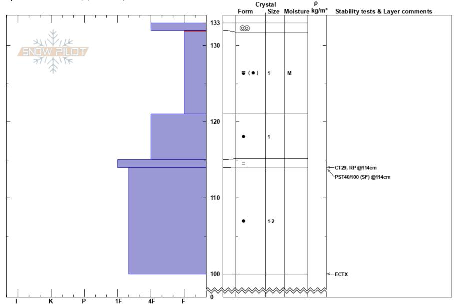
Notes: Pit dug in wind protected below treeline terrain specifically for a loaded PST on the surface facet layer. Using a 10 cm thick artificial slab constructed on the snow surface using disaggregated snow and allowed to sinter for 1.25 hrs, the tese scored Loaded PST 29/100 SF @ 133cm.
