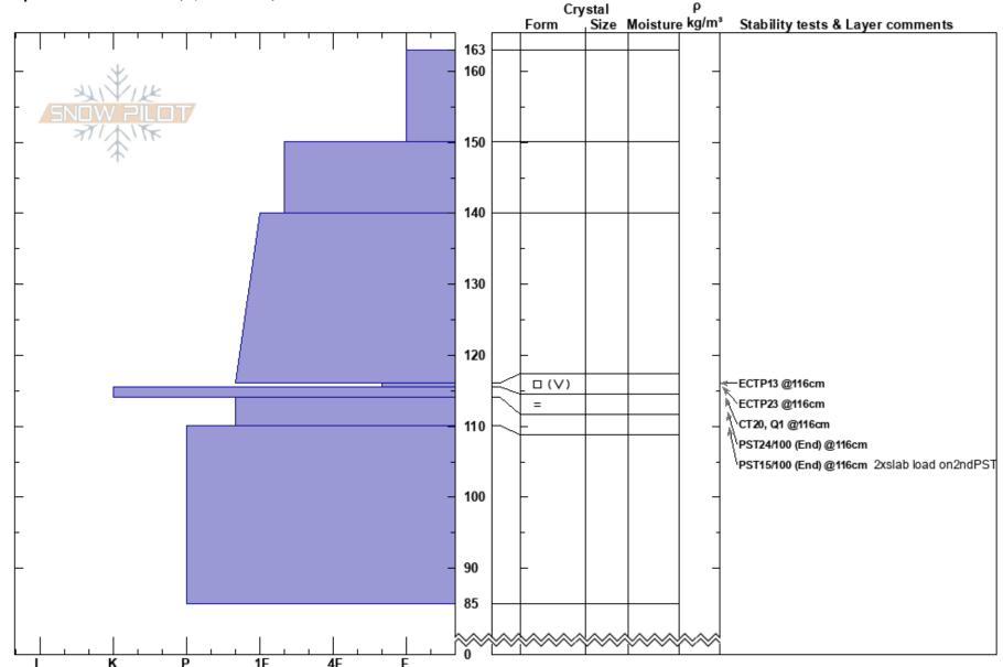
Notes: Prior pit to this lower on slope, at top of steeper meadow had ECTNs at storm interfaces, no propagation, or obvious SH layers. Weak layer was not obvious until CT, and then ECTP 13 was a bit of a surprise. Shorter PST cut (15/100) was result of placing slab from previous test on top of the second PST, essentially doubling the load.
