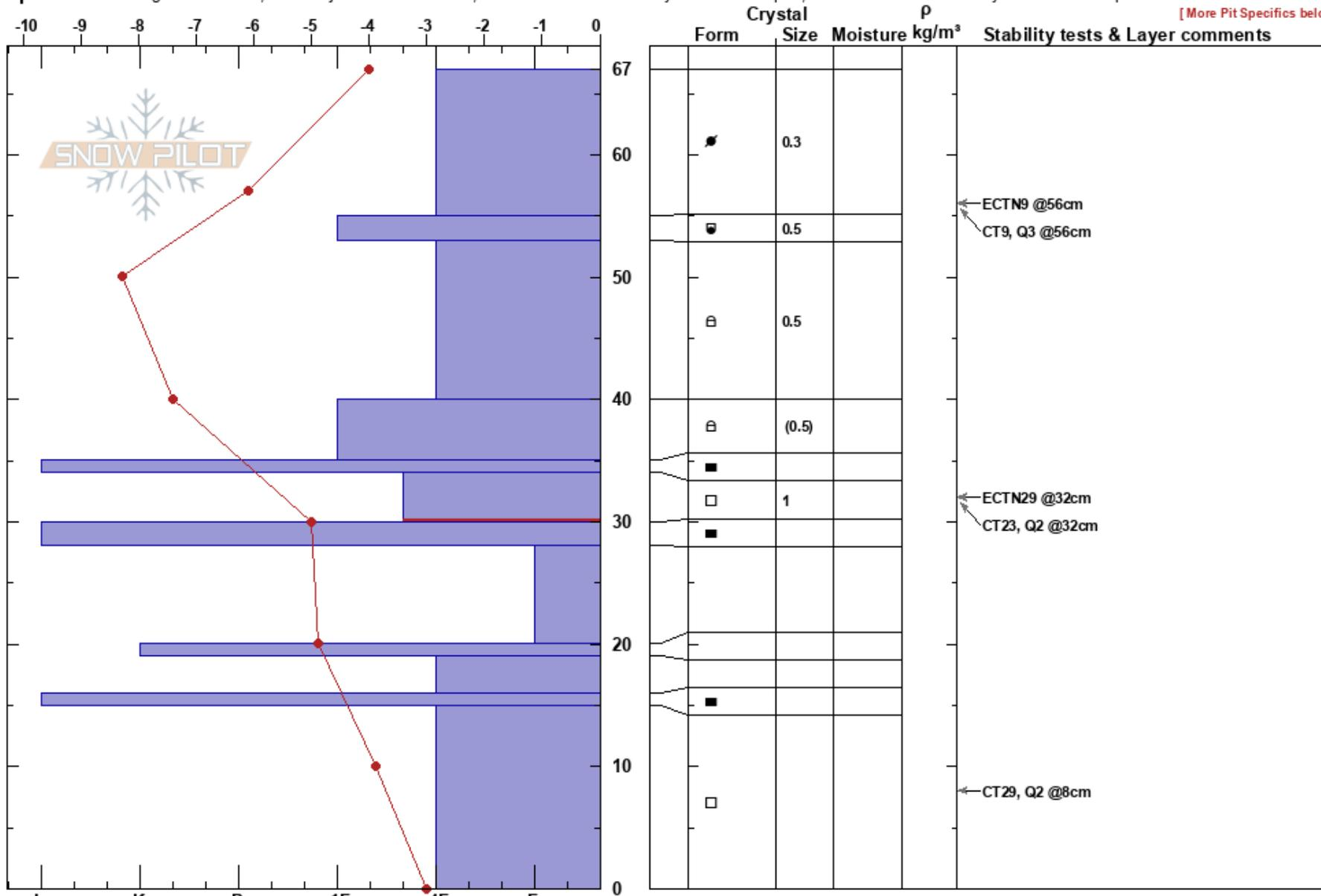
Notes: This pit was dug on the left side of Lenin, where it did not slide. It was hard to get crystal types because of the wind. Snow structure still looks like crap, but the test scores make it seem stronger. Additional Pit Specifics: Ski tracks on slope; We skied slope
