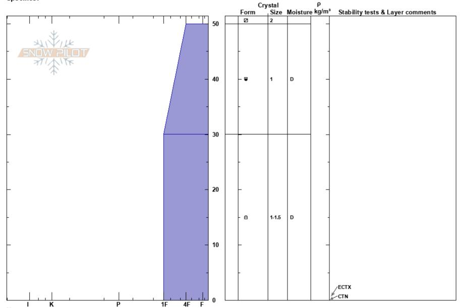
Notes: Some basal facets were visible in parts of the profile walls, but too isolated to include in this diagram. Snowpack tests targeted these areas, but did not produce any results.
