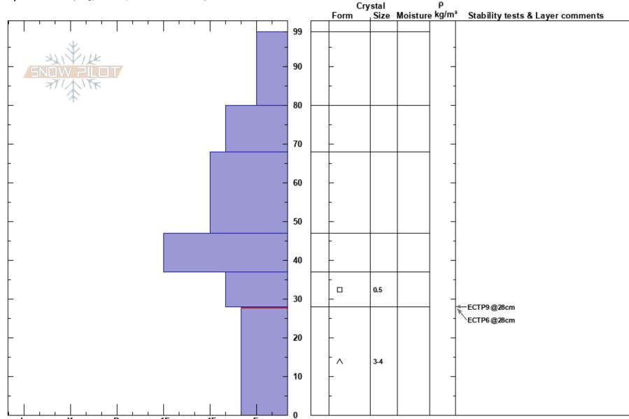
**Notes:** The slope may have collapsed when I approached on the sled. I couldn't hear it but saw a couple of saplings wiggle and drop their snow. Also, weak layer at 28 cm collapsed about 6-8 cm when the ECT failed.
